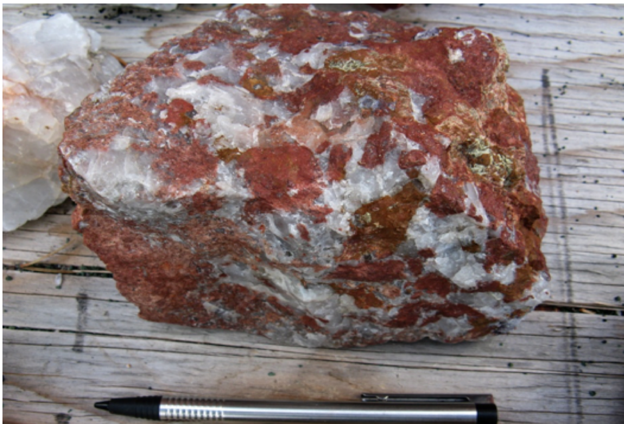
Figure 3: A sample of North T mineralised ore. Rare earths are contained within the red bastnaesite minerals and white material is quartz waste rock. Vital intends to initially separate the bastnaesite materials via conventional ore sorting technology.
