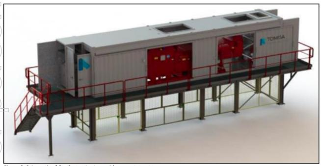
Figure 8: Schematic of Ore Sorter, in place with support structure.
