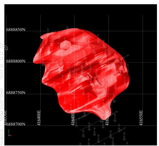
Figure 5: Plan view showing the 3D geology wireframe for the North T-Zone Bastnaesite Subzone
