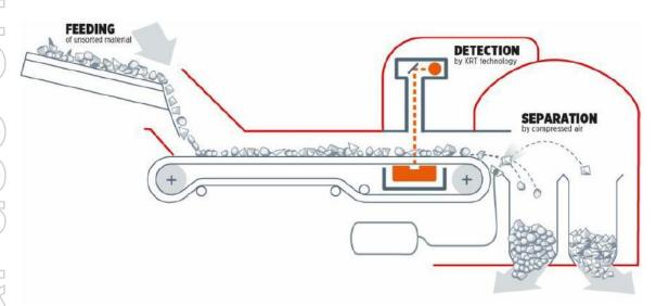
Figure 7: Schematic of Ore Sorting Process
