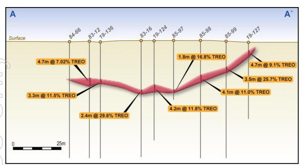
Figure 3: A typical long section through the Bastnaesite Subzone showing high grade intercepts
